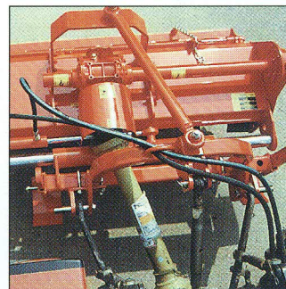
Although the gearbox is fixed in the machine very good PTO angles can be achieved in any position.
