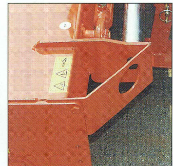
The profile of the right side has been designed to avoid damage to lower branches..
