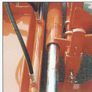
The hydraulic cylinder provides smooth side movement of machine.
